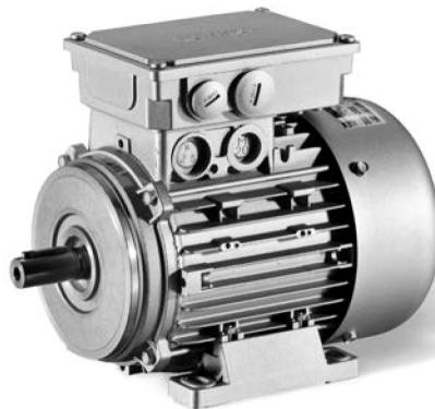
L-force MH three-phase AC motors are available in a power range from 0.75 to 45 kW and comply with efficiency class IE2 (high efficiency) as per IEC 60034-30.
